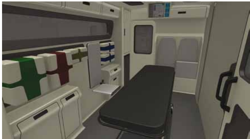
A computer-generated rendering of the proposed ambulance interior, with the stretcher repositioned to the middle of the treatment space
