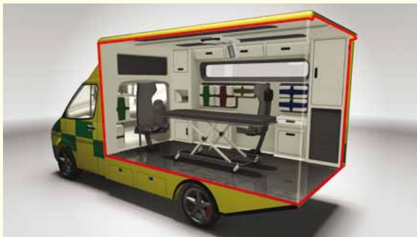
A computer simulation showing the proposed new layout, including the "working wall" and central stretcher
