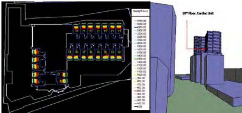
Figure 6 (above): Daylight simulation with a full progressive radiosity inter-reflection method
