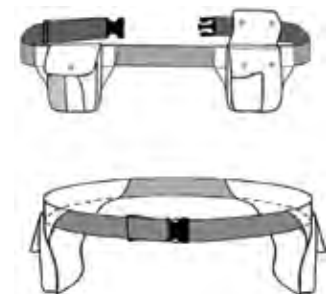
Figure 6: Concept for external carrying and storage object positioned at the waist or hips with different compartments. Above: opened buckle, back view. Below: closed buckle, front view
