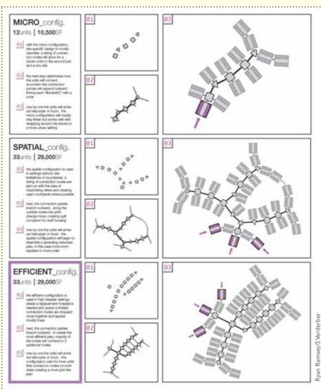
Figure 5: Suggested configurations for the prototype, according to site limitations and level of disaster
