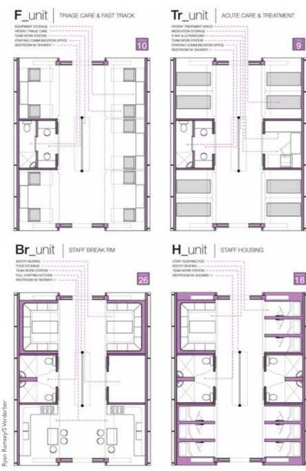
Figure 6: Internal configurations can be adjusted according to need – from surgery space to staff housing
